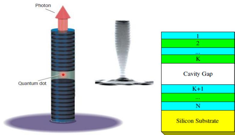
Figure 1: Scanning electron micrograph of a Fabry-Perot micropillar cavity [2] and a schematic diagram of a Fabry-Perot microcavity[3]
